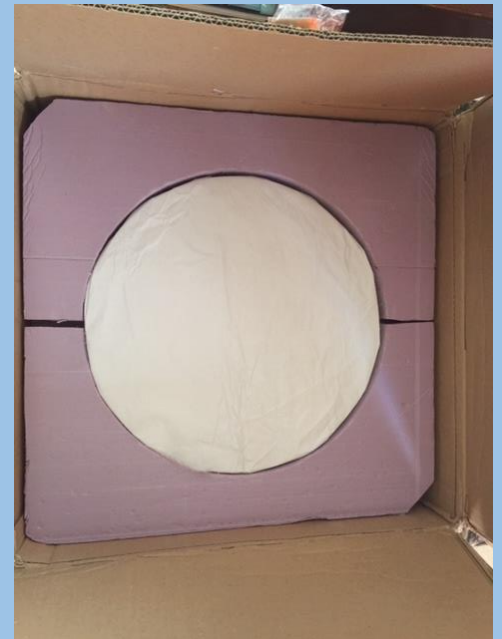
2" thick foam board cut circular for the mirror. I used a band saw, but a razor knife will work; it's just not as neat. Note how I cut the corners of the foam for ease of removal from the carton.
